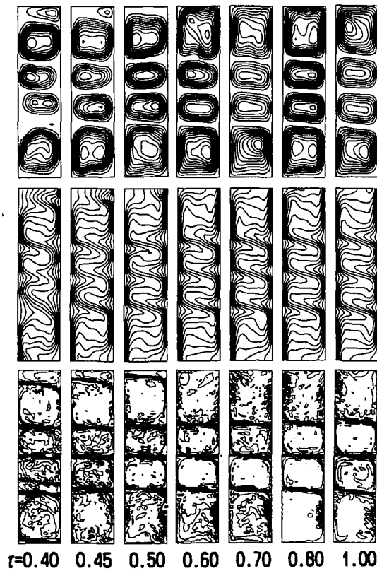
FIG. 6. Transient changes of the instantaneous contours of stream function (top row), temperature (middle row) and concentration (lower row) for Pr = 6 , Le = 100 , A = 4 , Ra = 10^6 and N = 10 .
